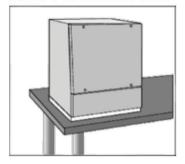
Closes off open bottom of sloped-front enclosures that are table-top mounted or suspended from overhead. Base is 14 gauge steel and has a ground stud provided. Foam-in-place gasket assures a water-tight and dust-tight seal. Steel bases are finished with RAL 7035 textured light-gray polyester powder paint. A top support bracket can be installed inside a 600-mm wide base for reinforcement when a COMPACT Pendant Arm Series 4 System 50, 60 or 80 is attached from below.
