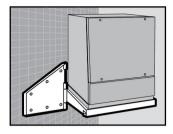
Hinged platform for a PROLINE sloped-front enclosure pivots 90 degrees from wall bracket, allowing complete access to rear of the sloped-front enclosure. The kit can be installed to pivot left or right and locks securely in position against a wall. Pivot pin is removable. Platform can support equipment weighing up to 300 lb. and includes holes to mount 600-mm wide sloped fronts in two positions. RAL 7035 textured light-gray polyester powder paint finish. Includes
